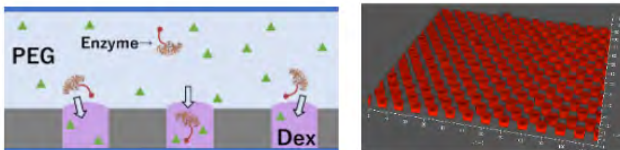
Fig. 2. On-chip enrichment system based on DEX/PEG ATPS. Schematic images of enrichment (left), and fluorescent image of DEX-rich droplets displayed on femto-reactor device (right)
